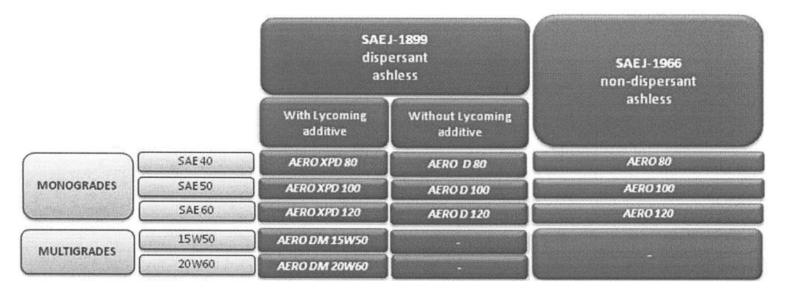
**TOTAL AERO XPD 80, 100, 120** oils are new generation ashless dispersive mineral monograde lubricants, developed to improve anti-wear and corrosion protection of piston engines.
