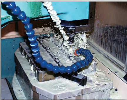
Machining pads at our facility
