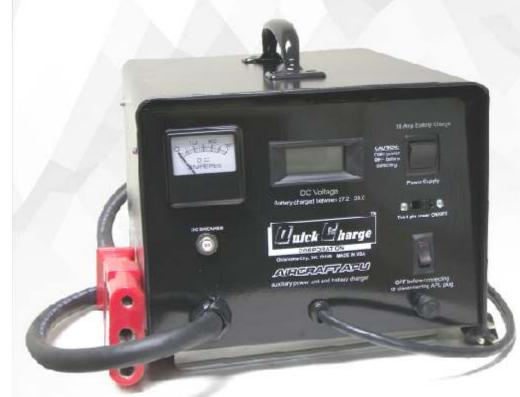
Designed to supply filtered DC bus power through standard APU receptacle in private and commercial aircraft. Up to 25 or 50 amp is available for operating avionics and flight control systems when the master switch is activated. Can also charge the battery through the plug at a 10 amp rate. Output is current limited, and will withstand starting loads. Voltage is limited to prevent battery overcharging.
