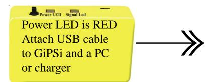
15 minute charge will run for one hour. 5 hours for full charge Note: Power Led is always Green during charging.
