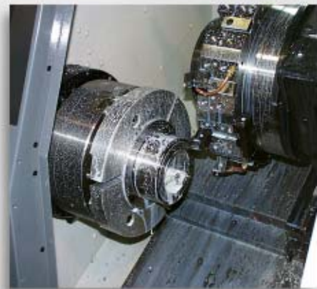
Each brake disc is 100% machined for increased strength and integrity
