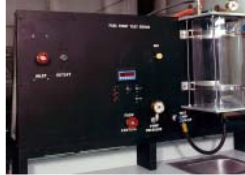
Fuel Pump Test Cell
