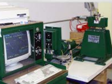
Each armature is computer balanced.
