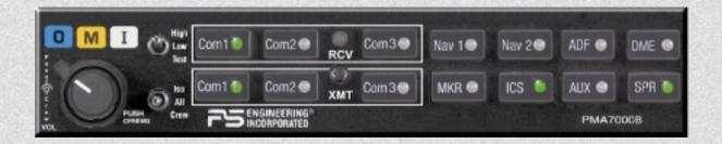
What do you do when you have the best audio panel in the world? You make it better! After nearly four years of production of the PS Engineering flagship PMA7000M-S, the company has rolled a number of product options into a new unit. Called the PMA7000B, this version incorporates the most requested features of the PMA7000M-S and PMA7000MS-CD.
