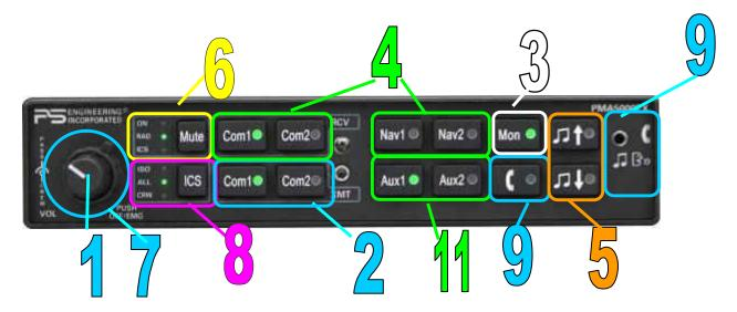
Figure 3-1 PMA5000EX Operating Controls
