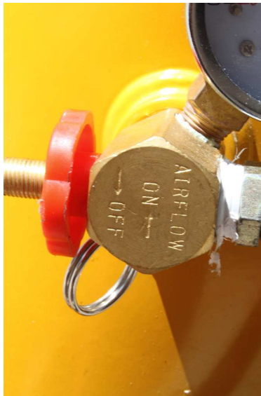
Figure 5: Air Tank Valve (must open to fill via quick connect)
