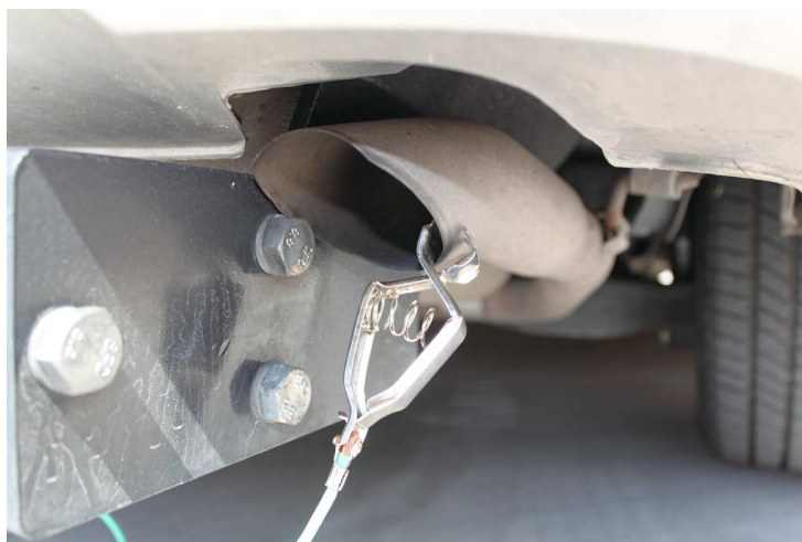
Figure 8: Attached Bonding Wire
