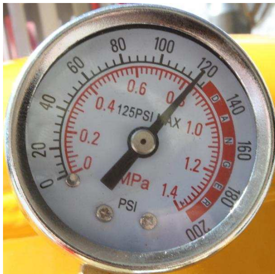
Figure 7: Air Tank Pressure Gauge (120psi)
