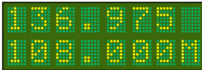
Monitor Mode Monitoring on STANDBY frequency
