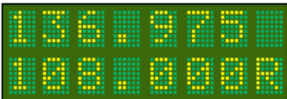
Monitor Mode Receiving on STANDBY frequency
