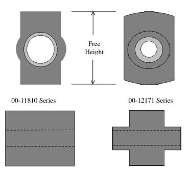
The picture above illustrates Barry Controls' molded spacers and their free height dimension. Table 2 at the end of this document will give the free height dimension for these molded spacers.
