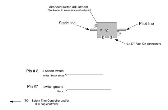
Note: Pin #7 is a common switch ground for all trim switches and the airspeed switch. An airframe ground may be used as an alternative
