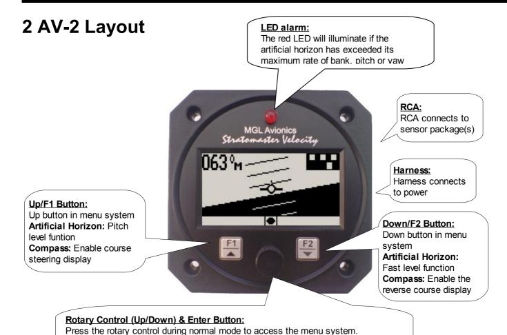
Rotate anti/clockwise for up/down menu scrolling. During normal mode turning the rotary control anti/clockwise will scroll through the main displays
