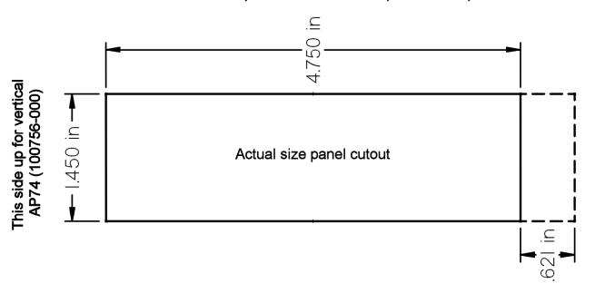
Mounting tab (in dashes above) can be match-drilled and secured to panel if
