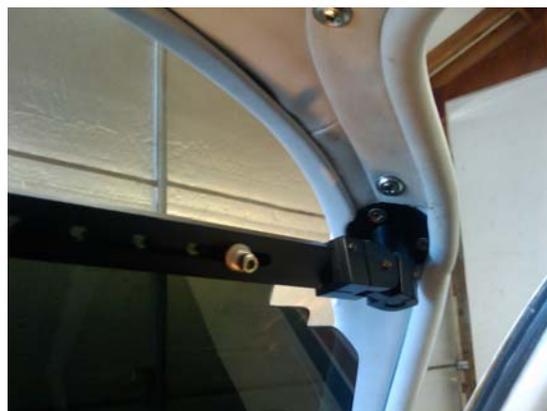
**Note: The 8-32 mounting screw is offset and will be on the lower side when installed.**
