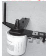
This tool was designed to eliminate much of the mess that occurs with small handheld oil filter cutting tools. Very simple to operate, it is excellent for individual aircraft owners as well as FBO's and maintenance shops where a lot of filters need to be cut. Simply clamp in a vise, screw on the filter, turn the cutter into the filter and hand crank to open the filter. The rugged construction enables this tool to operate trouble free for years.
