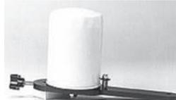
This aviation oil filter cutter will open any size oil filter canisters for your inspection. To use the tool, place the filter in a vice, attach the tool to the top of the filter, and rotate 4 to 6 turns to open the canister. The cutting wheel will stay sharp for about 50 uses, and is easily replaced when dull.
