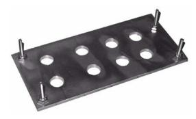
secure it. The long screws shown allow the servo to be raised and lowered simply by putting additional nuts on them so the servo is elevated above the plate. For a composite aircraft installation, the bottom of the plate (shown above) should be floxed and the holes in the plate filled with flox before applying fiberglass layers over it to secure it to the fiberglass structure.
