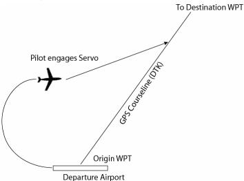
Note that the **SERVO LED** is now on and the autopilot has control of the aircraft.
