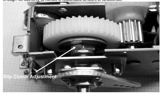
If you tighten the clutch enough to exceed the 30 in-lbs maximum torque rating, you may hear a loud clacking sound in the servo and the servo may disengage. This clacking happens when the force pushing the gears apart exceeds the solenoid's ability to hold the gear train engaged. This is a redundant safety feature – just back off on the control nut a little and recycle the power switch to re-engage the servo.
