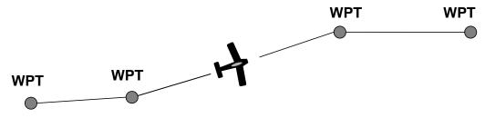
**2. Course mode (CRS)** – provides vector navigation as illustrated below. **CRS** also allows tracking an autopilot-selected course when the host GPS route function is not in use. **CRS** mode uses the GPS signal to provide the aircraft groundtrack. This mode can be useful for avoiding restricted airspace, weather and oncoming air traffic.
