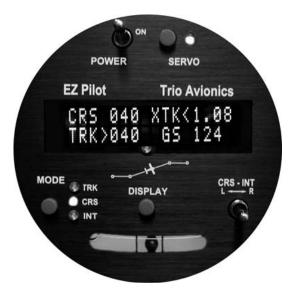
Going directly back to the TRK mode causes the EZ Pilot to more gradually curve back to the DTK.
