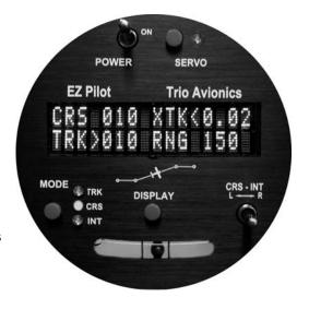
**NOTE**: If **SERVO POWER** is turned on (cycled) while in the **CRS** mode, the current track over the ground is automatically entered as the commanded **CRS**.
