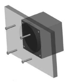
The EZ Pilot control head mounts from the rear side of the instrument panel. It is held in place by 4 ea. Number 6 screws. When mounted, the visible area is contained within a standard 3-1/8 inch instrument cutout.
