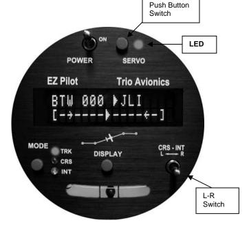
initial power up, the display will default to a flashing "NO GPS" message. In this condition the autopilot may still be used to provide a wing leveler function and the L-R switch can be used to initiate turns to the left or right. Once GPS data is present and validated, full navigation function is available.
