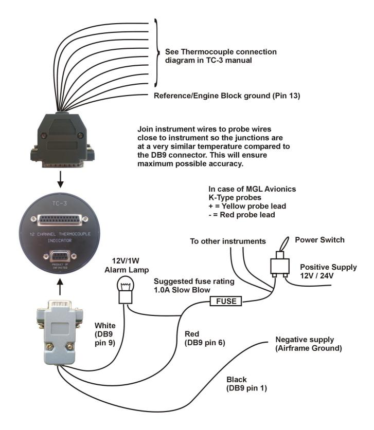
The use of an external 1A fuse is recommended. Connect the supply terminals to your aircrafts power supply. The TC-3 can be used on both 12V and 24V without the use of any pre-regulators. Ensure that the supply voltage will not drop below 8V during operation as this may result in incorrect readings.
