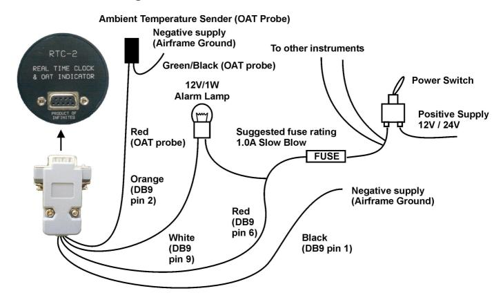
The use of an external 1A fuse is recommended. Connect the supply terminals to your aircrafts power supply. The RTC-1 can be used on both 12V and 24V without the use of any pre-regulators. Ensure that the supply voltage will not drop below 8V during operation as this may result in incorrect temperature readings.
