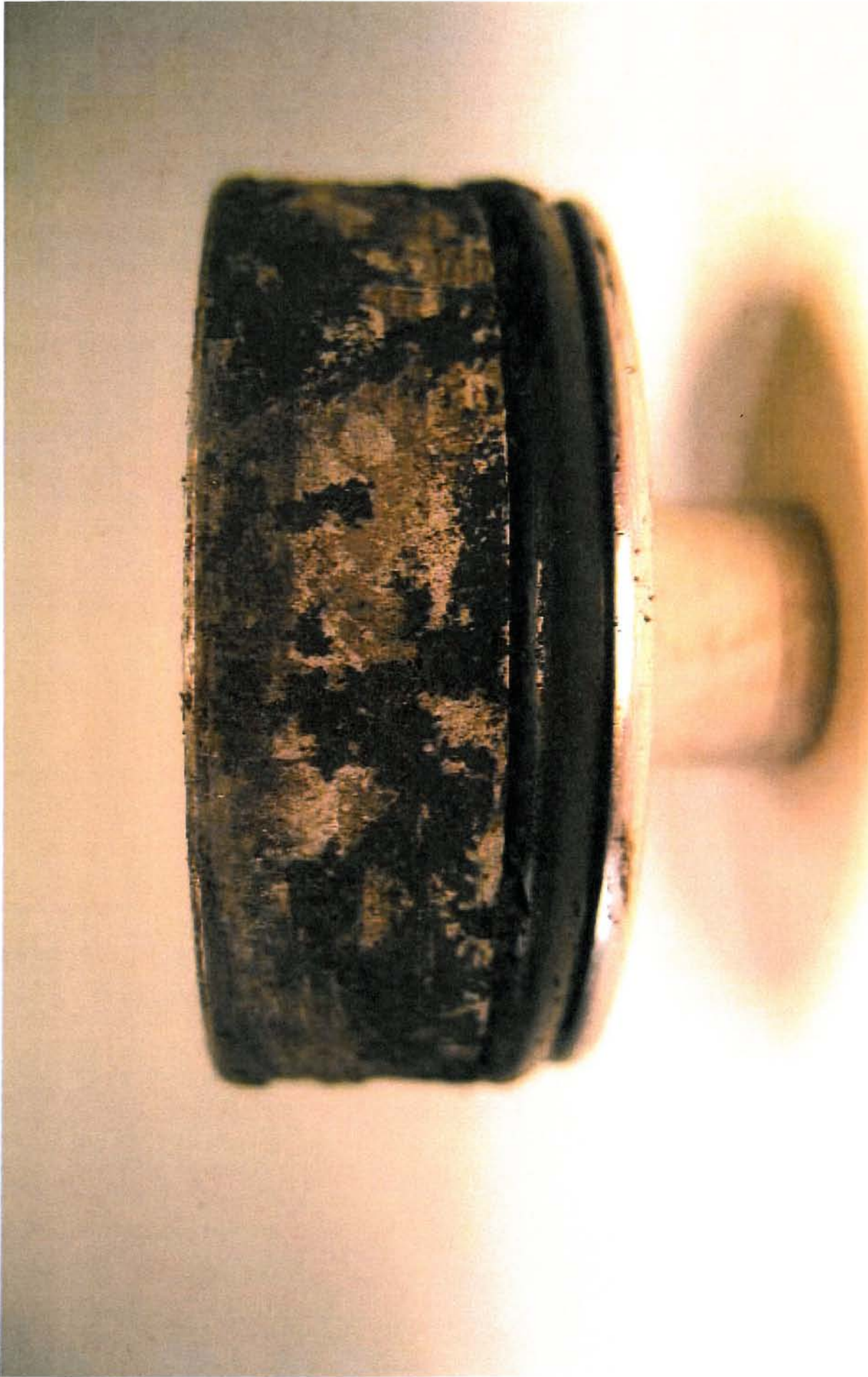
Dirty pistons stick and cause excess wear of linings, and over temping of disc.
