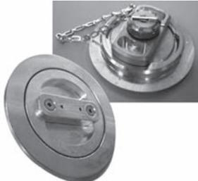
The ACS Twist-To-Lock Flush Fuel Cap Assy is machined from 6061 aluminum billet. The cap is available in vented and non-vented configurations. The sealing element for the cap is an easily replaceable viton "O" ring. The bottom of the cap is secured to the bottom of the ring by a safety chain to prevent loss of the cap during flight. The mounting ring may be welded, riveted, bolted or molded onto the tank.
