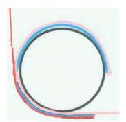
transition of vertical fin to top of fuselage skin are permissible without a sewed seam. A minimum overlap seam of 1" is required with a minimum width of 2" finish tape centered over the edge of glued seam.
