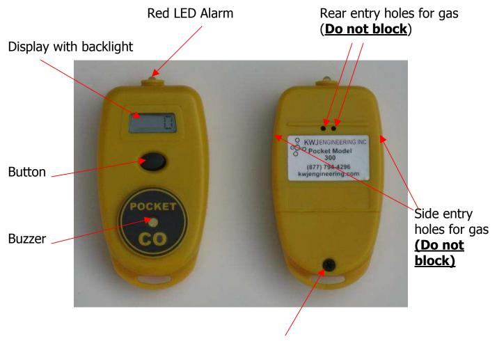
Screw for battery compartment cover
