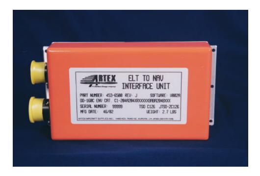
The Artex "ELT to NAV Interface" is designed to connect between the aircraft's Flight Management Computer (FMC) or GPS receiver and Artex' 406MHz series of ELT's. Its function is to receive continuous position updates from the aircraft's navigation system and translate it to the proper format for use by the ELT. Upon activation, the ELT transmits the Latitude and Longitude of the aircraft to the COSPAS/SARSAT
