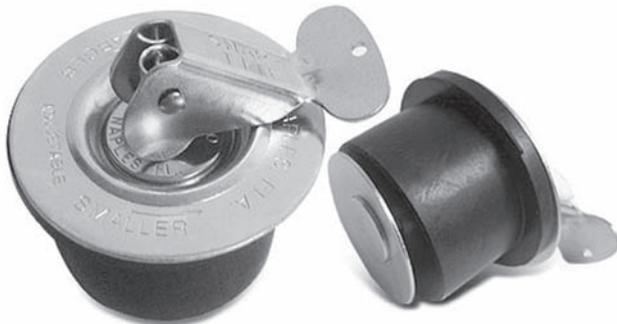
Pressure fuel caps are recommended for aerobatic installations. These caps are made with Buna-Nitrile gaskets for fuel resistance. These caps are non-vented for gravity fuel systems. It is highly recommended that a #40 (3/32") drill is used to drill a vent hole through the lower base plate and stud assembly using a drill press.
