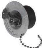
The 2 inch Piper PA-23 fuel caps are back. PMA Products, Inc. announced the return of their CA17672N fuel caps that are manufactured with improved rubber specifically formulated to prevent swelling. This part number replaces Piper part numbers 454-084 and 17672-000. Specifications: FAA-PMA Approved. Eligible Aircraft: Piper PA-23 (Beginning S/N 23-1, Ending S/N 23-1182) Piper PA-23-160 (Beginning S/N 23-1177, Ending S/N 23-2046).
