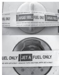
While most FBOs do a great job of keeping fuel orders straight, mistakes can and do happen. As for pilots, sometimes it's not feasible to stand around waiting for the fuel truck to ensure the right fuel is being poured into the aircraft tanks. FuelTape is a highly durable, weatherproof masking tape that clearly indicates to the fueler which grade of fuel must be used. Simply tear off a piece and stick it over the fuel caps and you have a low-cost, reliable system to keep your tanks safe.
