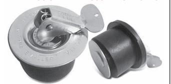
Pressure fuel caps are recommended for aerobatic installations. These caps are made with Buna-Nitrile gaskets for fuel resistance. These caps are non-vented for gravity fuel systems. It is highly recommended that a #40 (3/32") drill is used to drill a vent hole through the lower base plate and stud assembly using a drill pres
