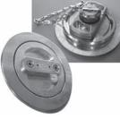
Assy is machined from 6061 aluminum billet. The cap is available in vented and non-vented configurations. The sealing element for the cap is an easily replace-able viton "O" ring. The bottom of the cap is secured to the bottom of the ring by a safety chain to prevent loss of the cap during flight. The mounting ring may be welded, riveted, bolted or molded onto the tank.
